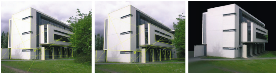
Fig. 3. An example reconstruction from a 200 frame video sequence. Two frames from the sequence are shown, with the reconstructed model overlaid in wireframe. The texture-mapped reconstruction is shown on the right from a different viewpoint. Total calibration time for this sequence was less than 10 min and model reconstruction took an additional 5 min.
