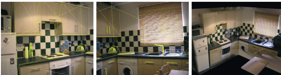
Fig. 5. A reconstruction from a pan/tilt/zoom video sequence. Total calibration time for this sequence under 10 min and model reconstruction took an additional 10 min.
