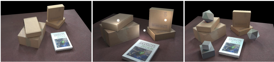
Figure 15: A reconstructed scene rendered from a novel viewpoint (left), with synthetic light sources illuminating the surfaces (middle), and with additional synthetic objects (right).
